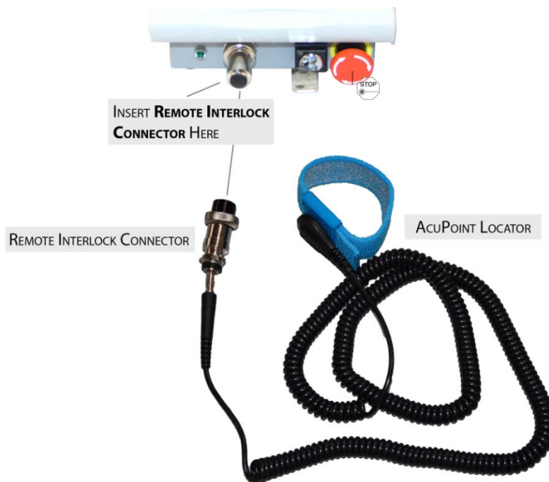
Figure 15. Wrist strap and connection to the TLC-1000 Laser Controller
